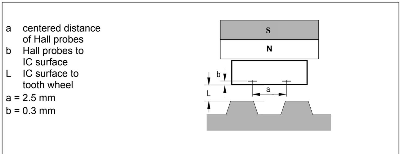
**Figure 6 Sensor Spacing**
