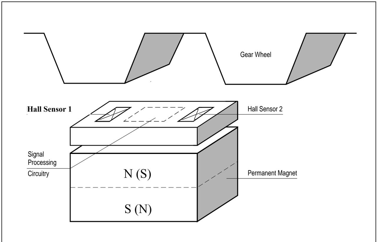
**Figure 8 TLE4925/TLE4925C, with Ferromagnetic Toothed Wheel**
