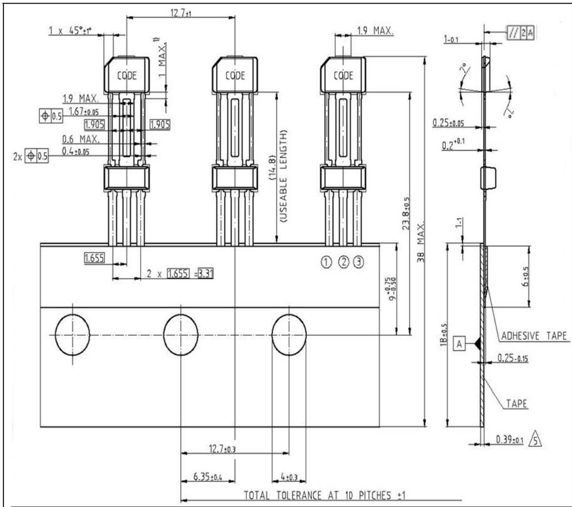
Figure 17 Tape Loading Orientation in the PG-SSO-3-9 package
