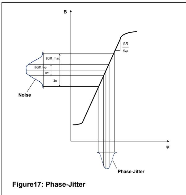
The phase jitter is normally caused by the analogue system noise. If there is an update of the offset-DAC due to the algorithm, what could happen after each tooth, then an additional step in the phase occurs (see description of the algorithm). This is not included in the following calculations. The noise is transformed through the slope of the magnetic edge into a phase error. The phase jitter is determined by the two formulas:
