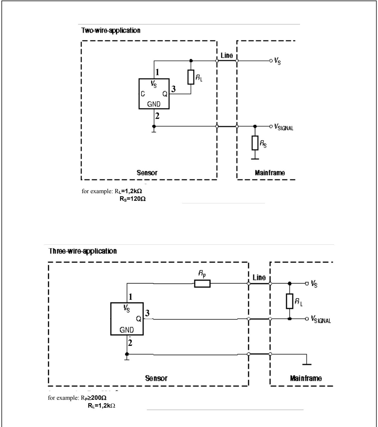
**Figure 10 Application Circuits TLE4925C (capacitors added in package)**
