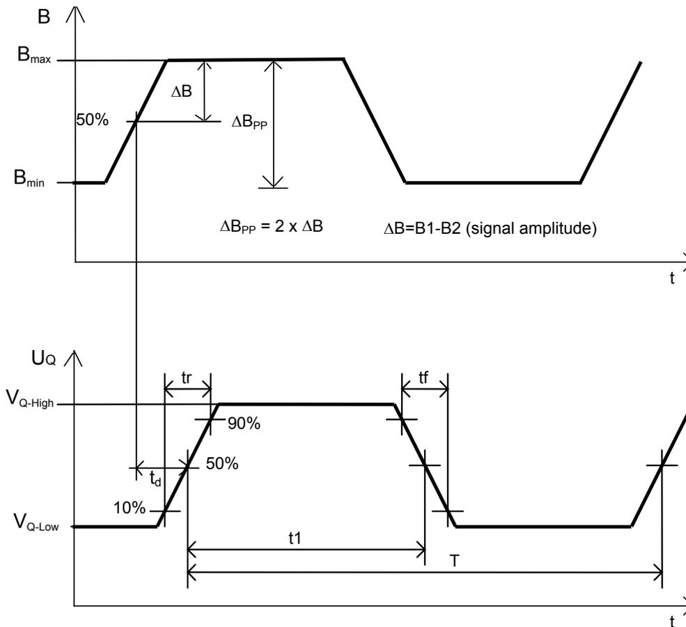
**Figure 4 Switching direction**
