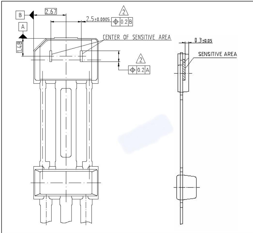
**Figure 16 Hall probe spacing in the PG-SSO-3-9 package**
